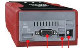
VGA Port Rotary Switch microSD Socket USB Client
